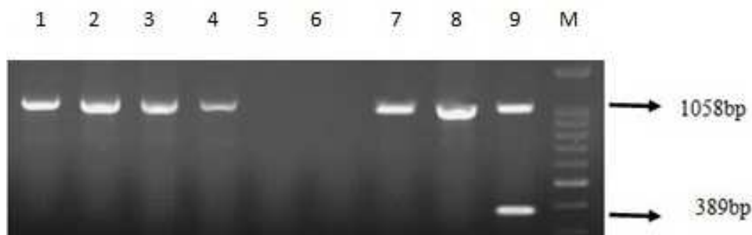
Fig. 3. PCR amplification fragments for the detection of oxa-23 and oxa-48 genes among Acinetobacter baumannii isolates. Lane 1- 4 and 7, 8: positive oxa-23 strains, lanes 5, 6: negative control of oxa-23 and oxa-48 genes, lane 9: positive control of oxa-23 and oxa-48 genes and M: 1kb DNA size marker
