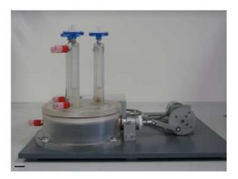
**Fig 4.** Pulsatile bioreactor. Comparison of different media, cells and scaffolds are enabled by three media compartments at defined mechanical loadings. Core unit manufacturing from acrylic glass provides optical transparency for macroscopical observation of processes within the unit (122). Scale bar = 20 mm.
