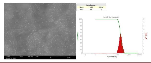
**Fig. 1.** Morphological and size characterization of CsNPs. SEM images depict CsNPs as generally spherical and uniform, with an average size of 144±12.8 nm. DLS analysis reveals an average particle size of 182.4 nm and a zeta potential of approximately +49.2 mV.
