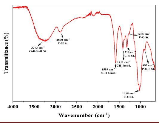
**Fig. 2.** FTIR spectrum of CsNPs. The FTIR spectrum of CsNPs shows characteristic absorption bands, including N-H and O-H stretching vibrations, C-H stretching vibrations, N-H amide bending, CH<sub>2</sub> bending, C-N and N-H amide vibrations, -C-O-C stretching vibrations, P-O stretching vibrations (shifted due to chitosan interactions), and P-O-P stretching. These features differentiate pure chitosan from chitosan-TPP.
